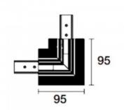
Busbar corner connector for finishing. Use together with Powergear L-shaped connector.
