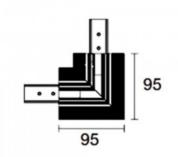
Busbar corner connector for finishing. Use together with Powergear L-shaped connector.
