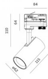
Three-phase track system adapter for GU10 bulbs An adapter designed for a three-phase track system, operating on a 230V power supply. It is compatible exclusively with GU10 bulbs, providing a simple and efficient lighting solution. Light sources are not included, allowing you to select the bulb that best suits your needs. A reliable and practical choice for creating high-quality lighting!
