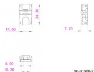
Connection clip for connecting two LED strips.
