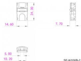
Connection clip for connecting two LED strips.
