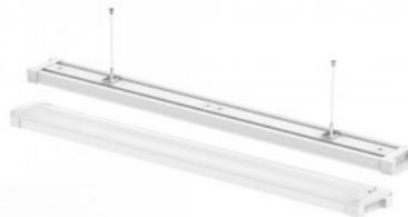
PROLUMEN Meena [linear luminaire](#) with adjustable power levels of 22W/30W/35W/40W. A high-quality linear light suitable for installation in parking garages, large closets, corridors, and warehouses. The Meena luminaire is designed to be very easy to install and maintain. The housing can be opened with a button press, and the suspension cables are adjustable during installation.
